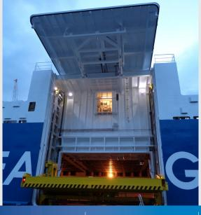
**CARGO CAPACITIES** Weather deck: Main deck: Lower hold: LM: 670 m 695 m 410 m 1250 m2 Deck area: 1920 m2 2150 m2 Height: 5.00 m 4,60 m Deck load: 3,0 t/m2 5,0 t/m2 5,0 t/m2 336 TEU Container capacity:
